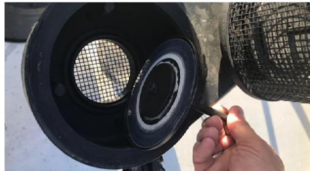
*PROSHIELD™ coated vent showing no signs of build-up after 10 months*
