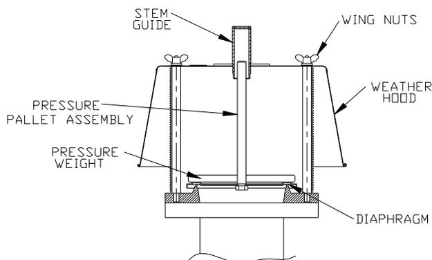
4. Check carefully to insure that all packing materials are removed from on or inside the vent housing and from the pallet assembly.
