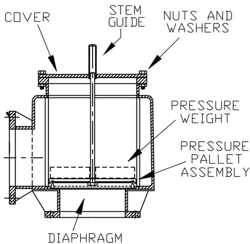
5. Mount the vent to the appropriate flanges using gaskets compatible with service conditions. For best performance, the vent should be mounted level so that the seating surfaces are no more than 1° off horizontal.
