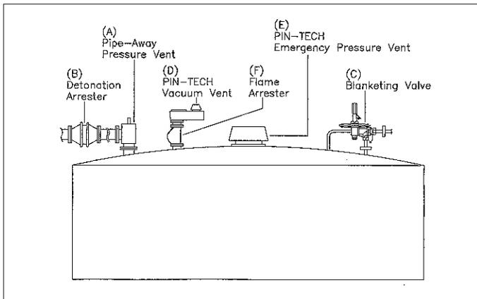
Normal pressure relief is provided through the Pipe-Away Pressure Relief Vent (A), with vapors directed to a destruction (flare) or recovery unit. The system is protected from possible ignition sources downstream by a Protectoseal Bi-Directional Detonation Arrester (B).
